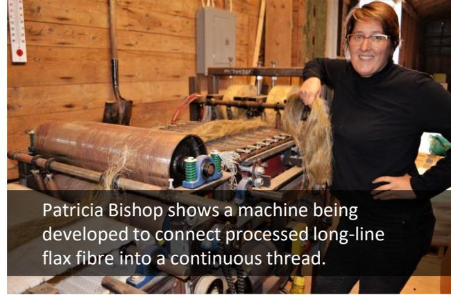
Patricia Bishop shows a machine being developed to connect processed long-line flax fibre into a continuous thread.
